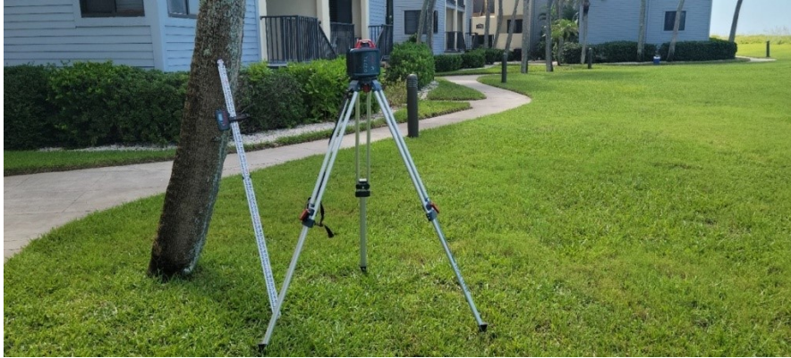
Self-leveling rotary laser level instrument kit with measuring rod.
