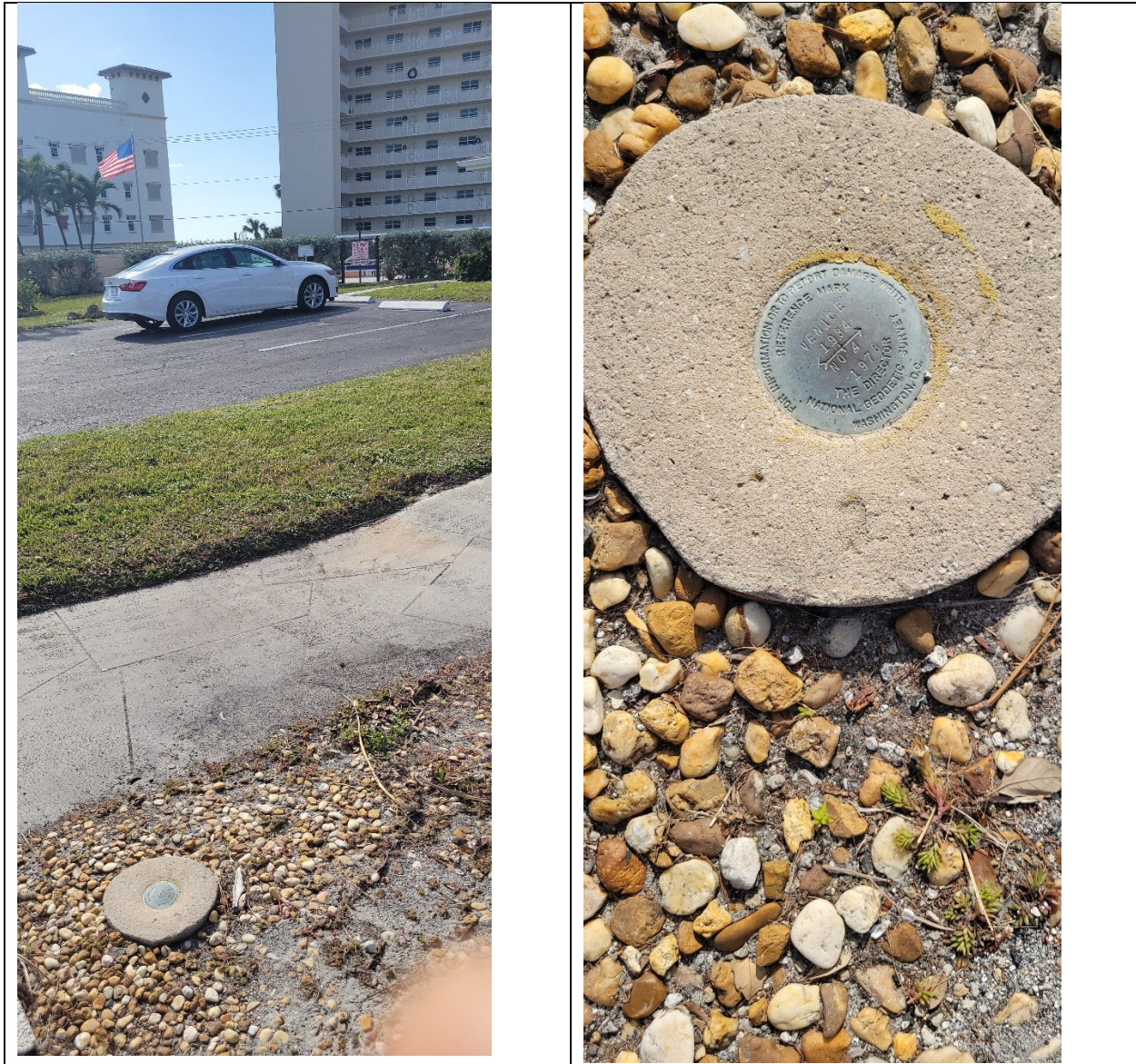
Benchmark plaque suitable for placing a measuring rod to determine height of instrument.
