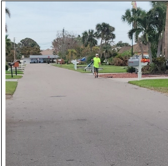
Leapfrogging the instrument to transfer established benchmark elevation to determine building elevation.
