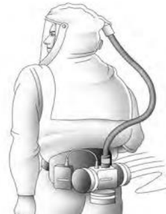
Hood Powered Air-Purifying Respirator (PAPR) APF= 25
