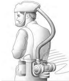
Loose-Fitting Powered Air-Purifying Respirator (PAPR) APF= 25
