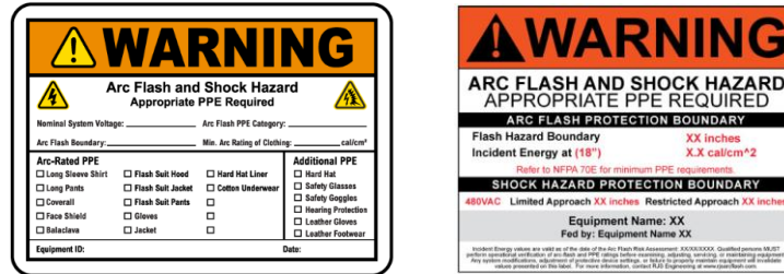
Figure 11: Category Label & Incident Energy Label
