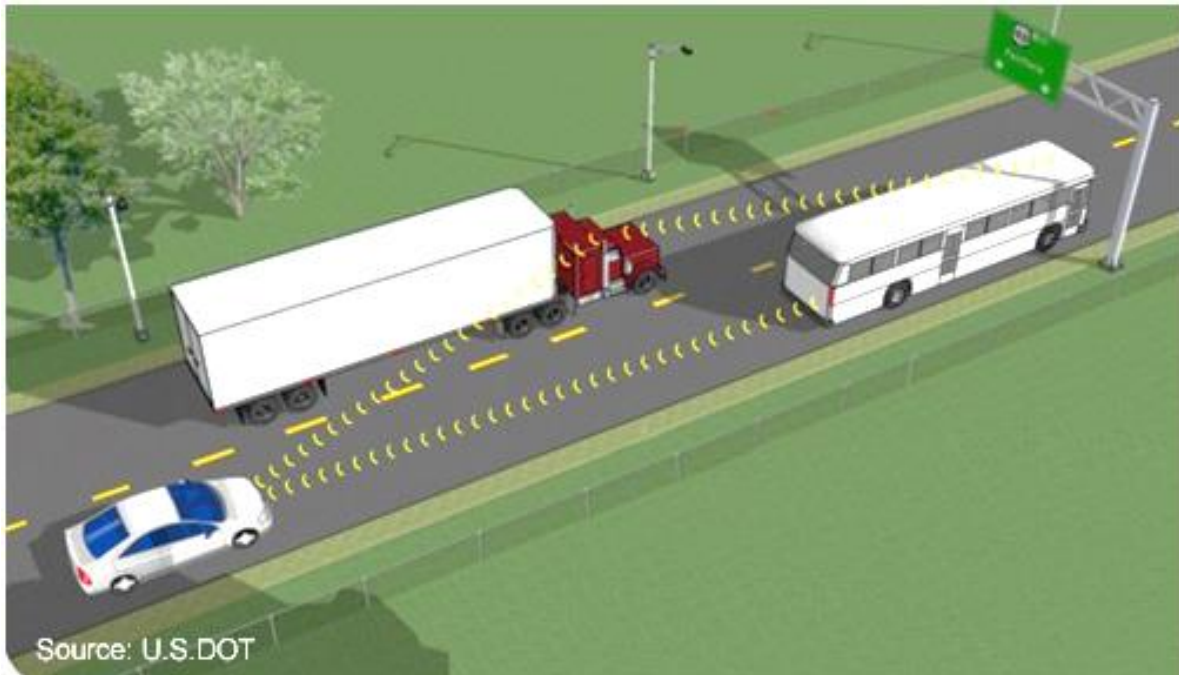
Figure 18: Depiction of vehicle to vehicle (V2V) communication as part of an AHS.
