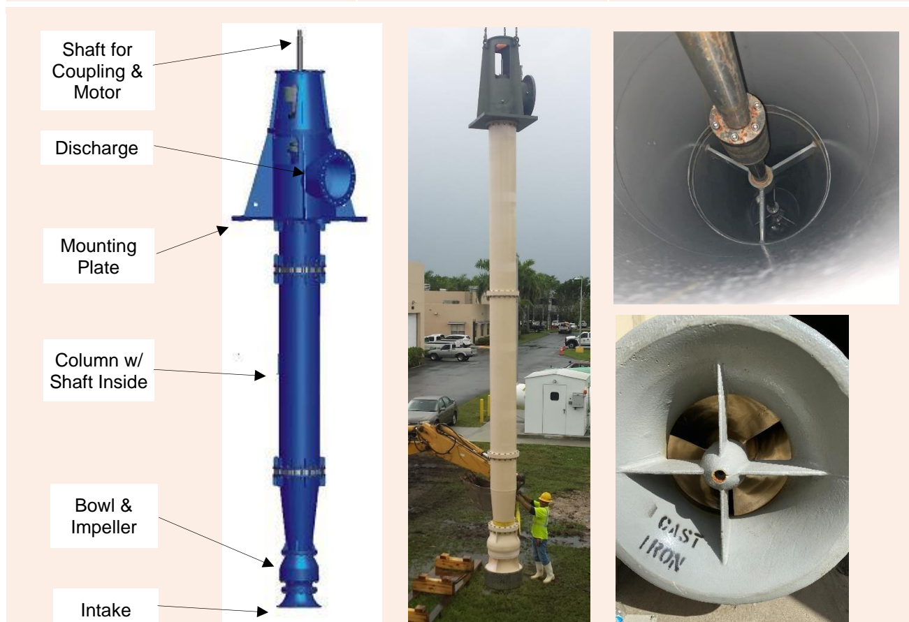
Figure 4: Left and Center: Example vertical turbine pumps. Upper Right: View looking down inside a mixed flow pump. The shaft is typically enclosed in a vertical turbine style pump for protection from corrosion and stringy material. Lower Right: Intake of a mixed flow pump with a bronze impeller.
