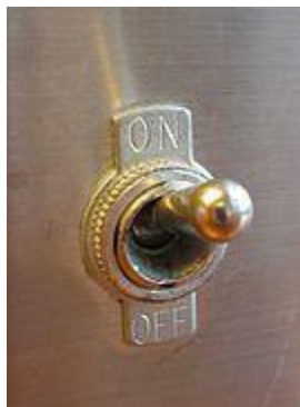
Figure 13: O/O hand switch (HS) on a control panel, with On and Off functions.
