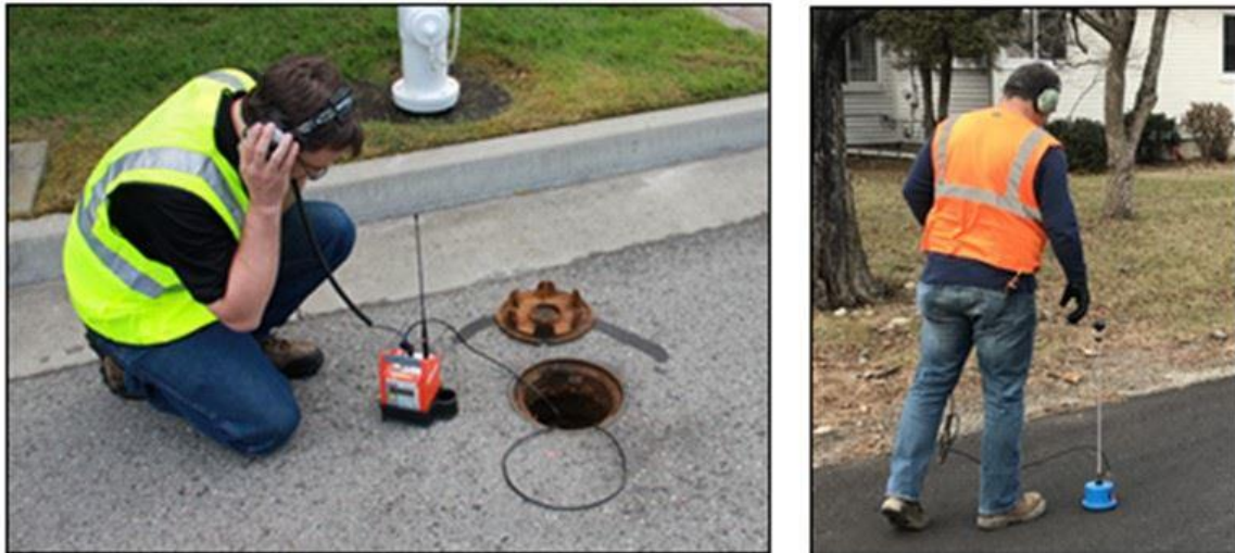
Figure 18: Technician using a correlator (left) and ground-mic (right).
