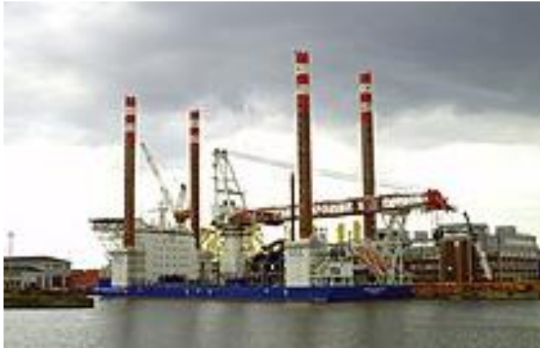
Figure 8: German Windfarm Construction Vessel. The blue part is the hull, and the crew can set the feet of the tall cylinder legs on the sea bottom and jack the vessel up the legs so it is above the sea. Note the worker accommodations to the left, a helipad on top, and a very large crane on the deck.
