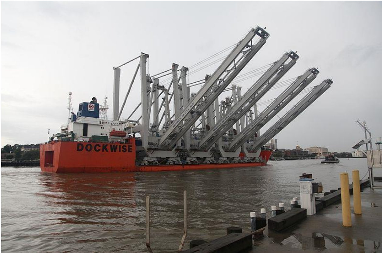
Figure 12: Another semi-submersible type carrying large container cranes to a port as cargo. How do they keep this from rolling over? See the course on Intact Stability to find out!
