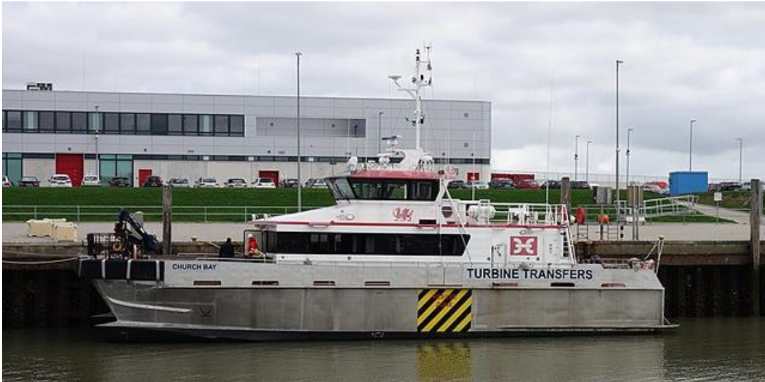
Figure 9. European Catamaran Windfarm Support Vessel. Note the wave piercing bow bulbs and raised foredeck crew transfer platform.
