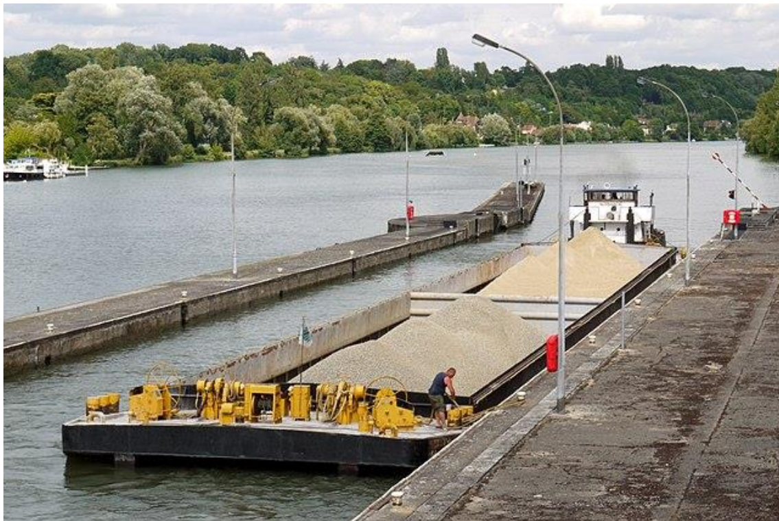
Figure 26: Pushboat and Hopper Barge with a load of gravel.
