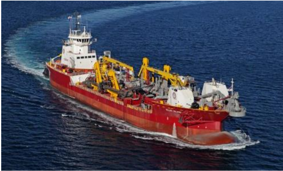
Figure 30: Trailing Suction Hopper Dredge (Courtesy of Eastern Shipbuilding Group)
