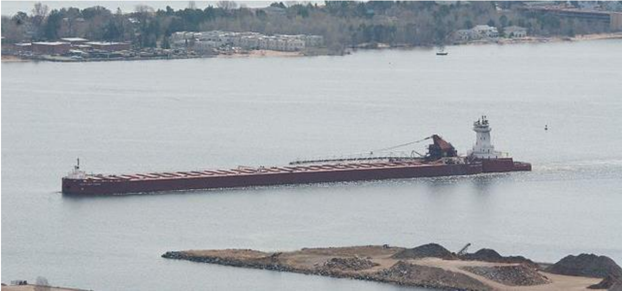
Figure 22: ATB Combination on the Great Lakes. The barge is a bulk iron ore carrier, built with a notch for the tug at the stern, and no engine room section for propulsion. The tug locks into the notch and acts as the engine room for the barge.
