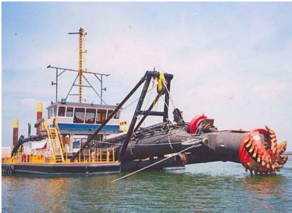
Figure 31: Forward Suction Conventional Dredge with cutter head up
