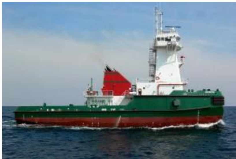
Figure 21: ATB Tug. Note the gray box on the side under the pilothouse-this is the pin device that connects the tug to the barge, and it locks the tug into the rolling of the barge but allows the tug to trim separate from the barge.
