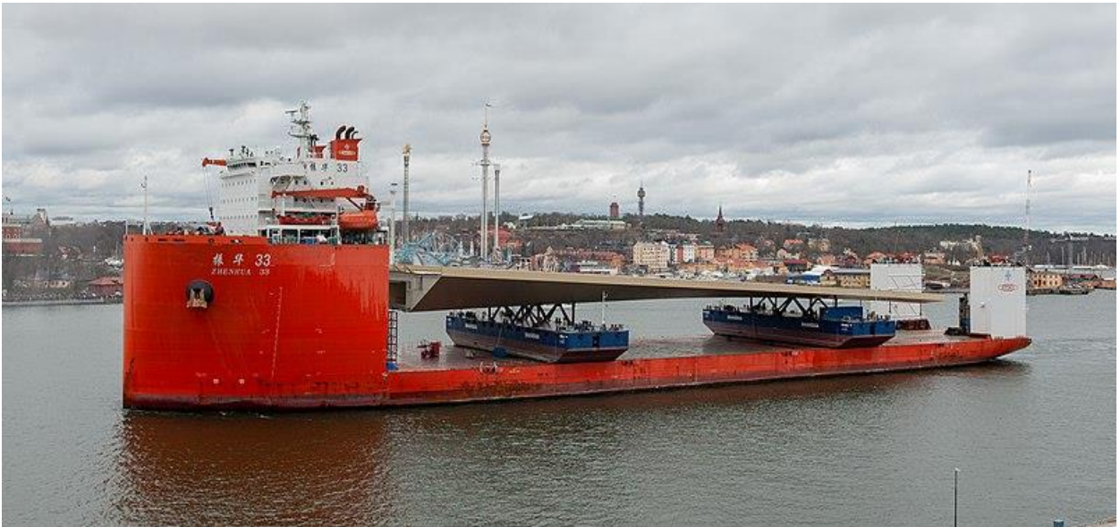
Figure 11: This is a semi-submersible heavy lift ship. Unlike the ship in Figure 10, this ship floods the ballast tanks in the hull so that the main deck is deep enough underwater for the
