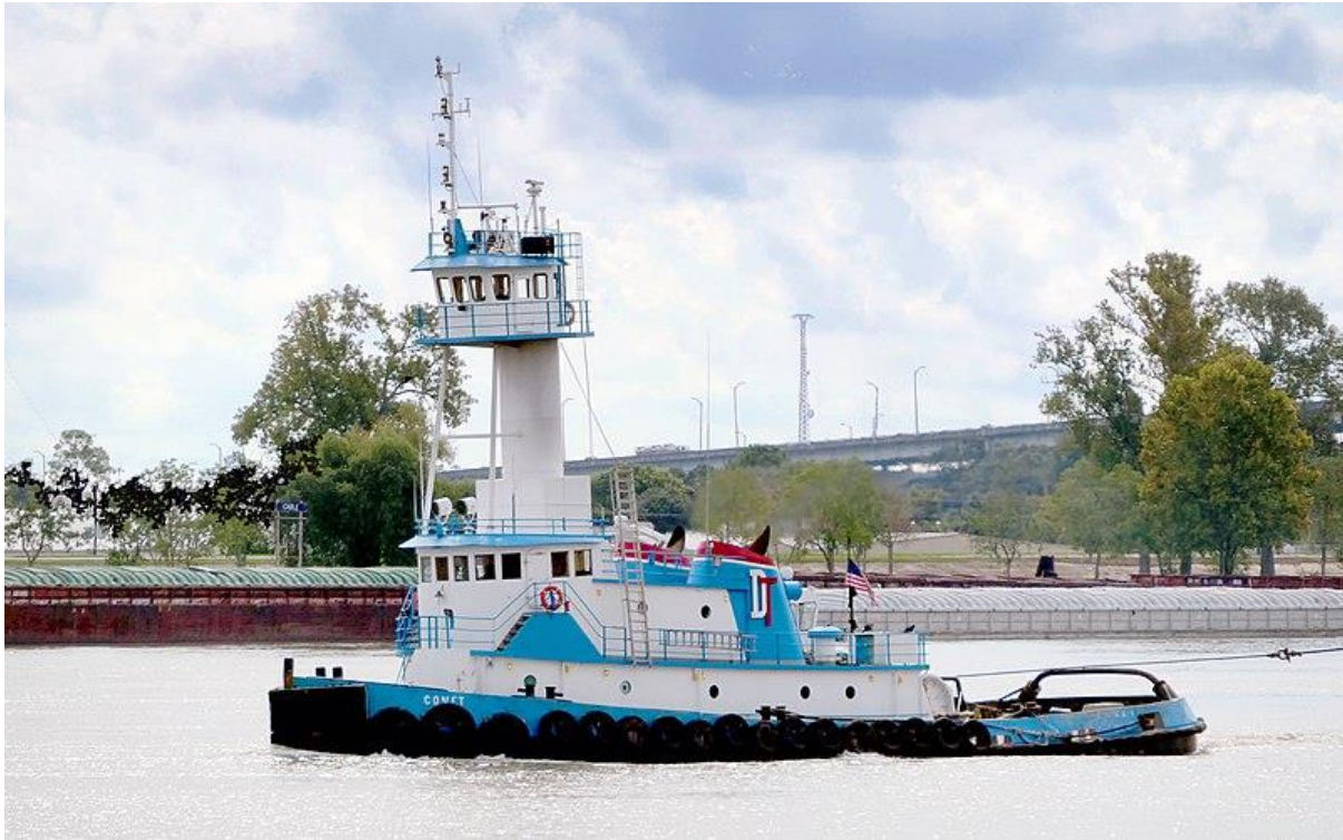
Figure 20: Convertible ATB Tug, in this case towing a barge behind it (see cable over stern). The person on the helm can steer from above or below depending on how much view is needed.
