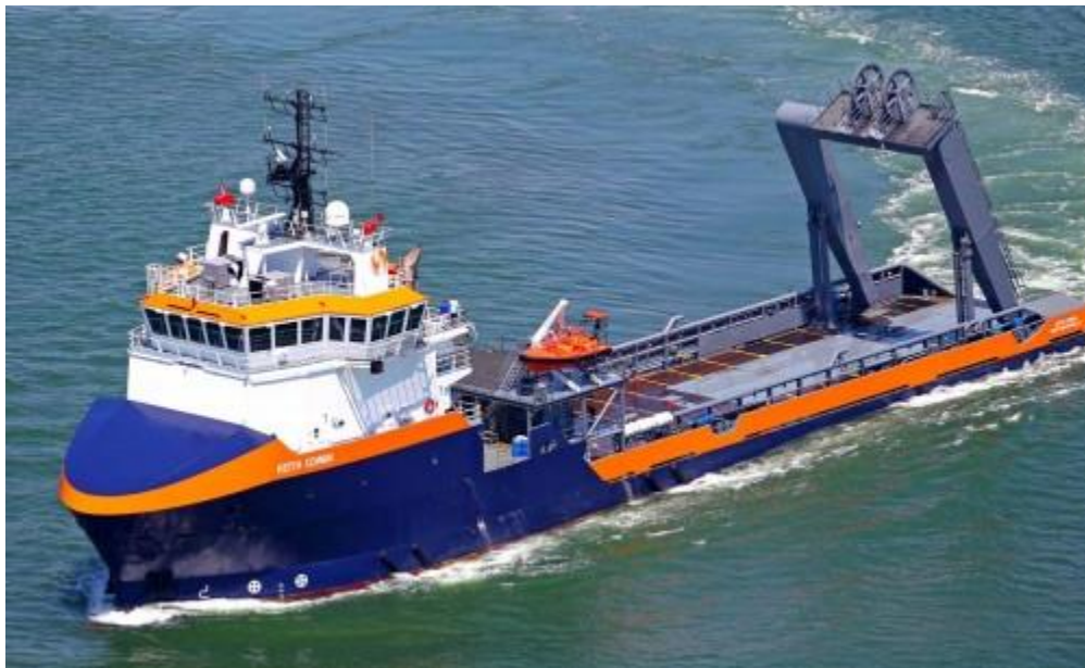
Figure 6: Anchor Handling Towing/Supply Vessel (courtesy of Eastern Shipbuilding Group)
