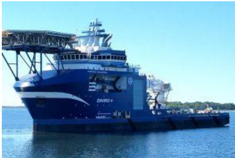
Figure 4: Platform Construction Vessel. Note large white crane on the aft deck and extra- large deckhouse for 72 crew and construction workers. The garage door on the side houses a remote operated vehicle. (courtesy of Eastern Shipbuilding Group)
