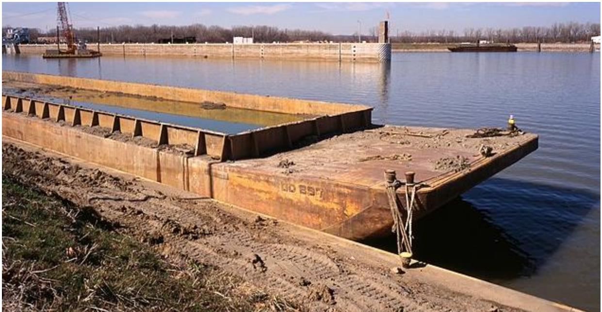
Figure 27: Deck Barge. The short wall on the deck is to keep the load in place and to fit a cover if needed.
