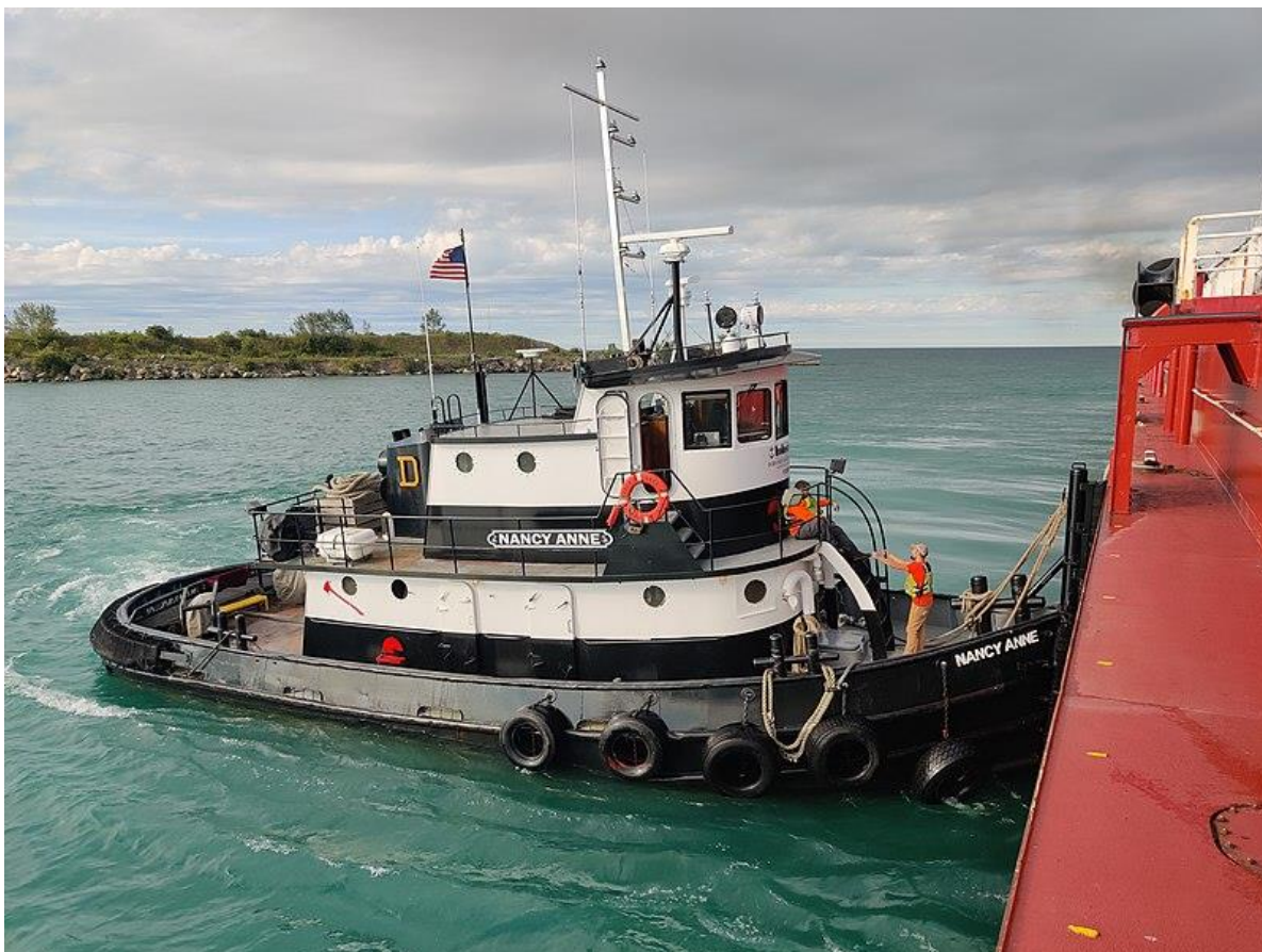
Figure 18: This is a typical “model bow” harbor tug of the older style propulsion.
