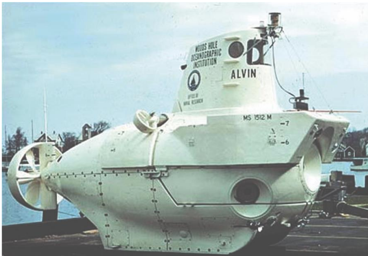
Figure 37: Manned Research Submarine Alvin (1980's period configuration when it found the Titanic)
