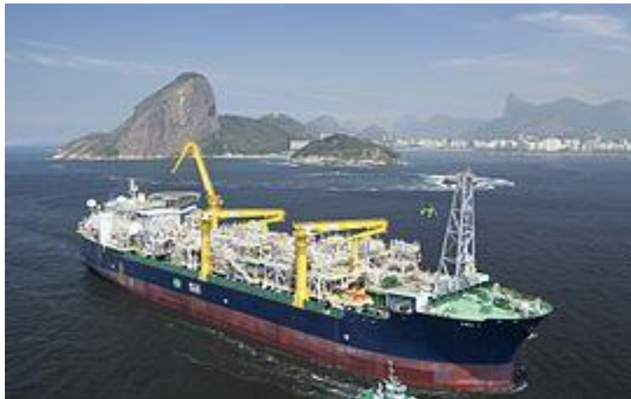
Figure 7: A tanker converted to an FPSO ship. An FPSO ship is similar to a tanker but it has additional piping and equipment on deck.
