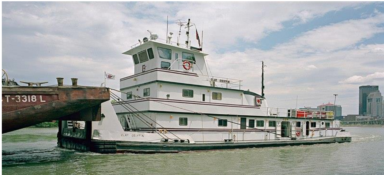
Figure 25: Pushboat pushing an unloaded deck barge. This is why the push knees are so high!
