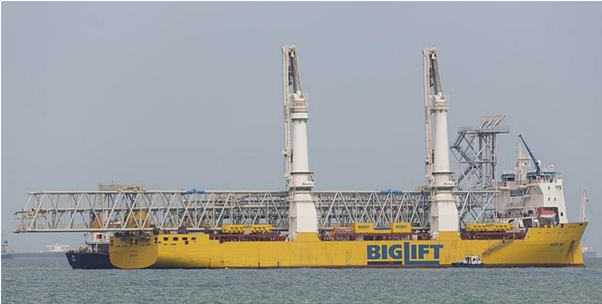
Figure 10: A heavy lift crane ship that carries large loads on deck. This cargo is the leg of a jack-up offshore oil rig.
