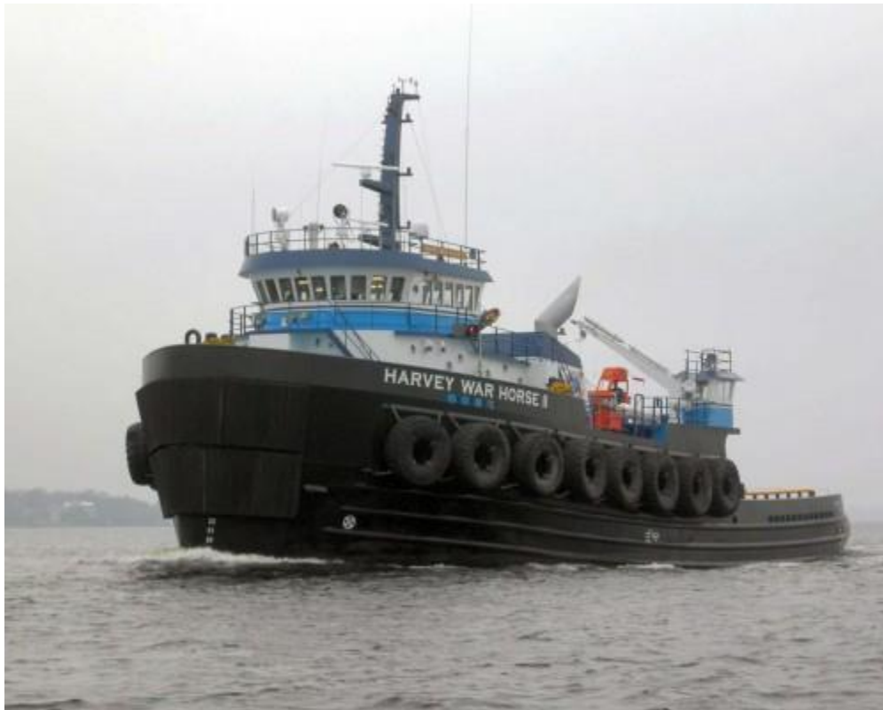
Figure 17: Seagoing Tug. Note the wide rubber padded bow for pushing, the high hull freeboard forward, the tires alongside for side towing and docking, the crane on the aft deck, and there is a large horizontal winch at the aft end of the superstructure (Courtesy of Eastern Shipbuilding Group)
