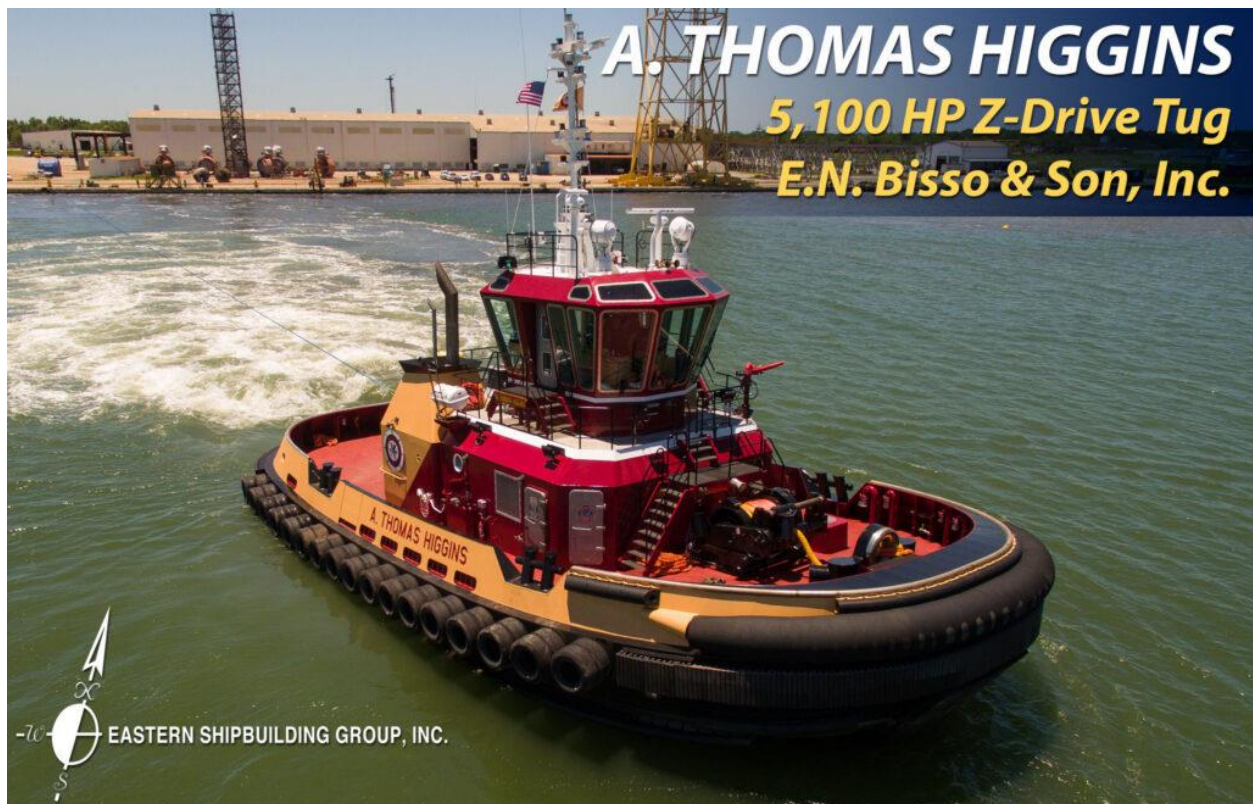
Figure 19: This is a newer style tractor tug. Note the superior all-around visibility in the pilothouse and the red gun to the right of the pilothouse-this is a fire monitor for fighting fires and it can spray a stream hundreds of feet. (Courtesy of Eastern Shipbuilding Group)
