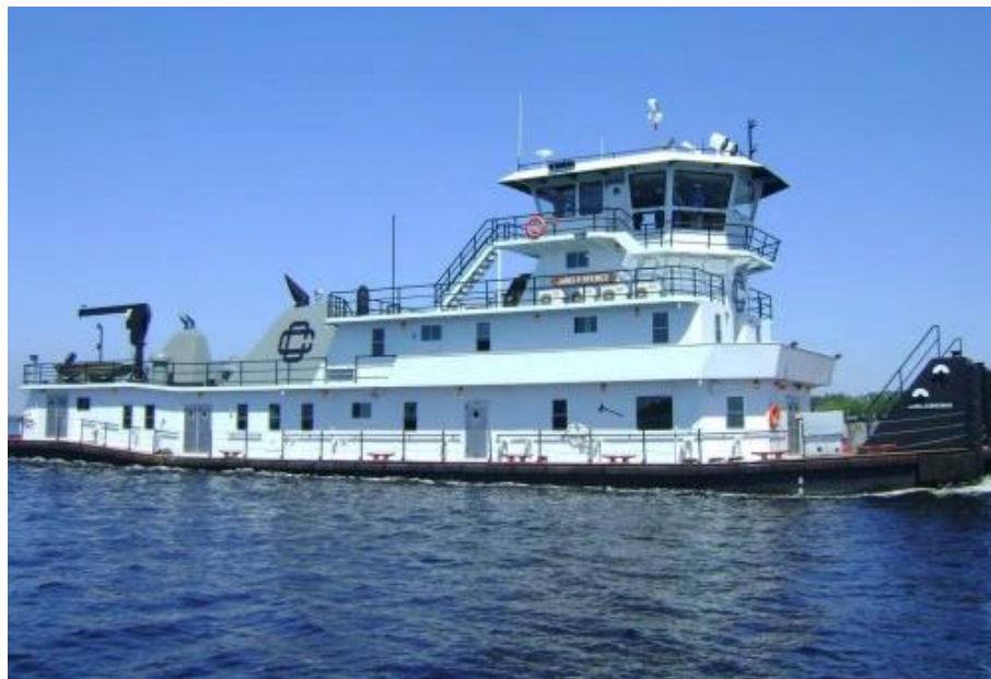
Figure 24: Larger, higher horsepower pushboat. This is typical of what pushes large groups of bulk material barges on the main rivers. My first marine job was as a summer intern at a shipyard that built these. (Courtesy of Eastern Shipbuilding Group)
