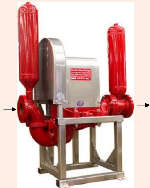
Figure 8: Left: Suction and discharge cycles of a double disc pump. During the suction cycle, the suction disc (on the left) rises and the clack valve opens to draw in fluid. During the discharge cycle, the discharge disc (on the right) drops to force out the fluid. Right: Example of double disc pump with vertical pulsation dampeners and 4-inch connections.
