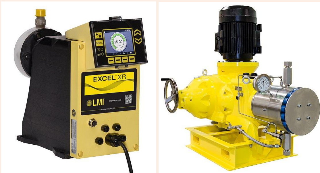
Figure 4: Examples of mechanically actuated diaphragm pumps. Left: Small metering pump with built-in speed control, control screen, and a standard outlet plug. Right: Large metering pump with a vertical motor designed for pressures up to 15,000 psi. The wheel is for manual stroke adjustment.
