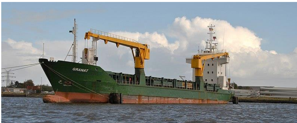
Figure 3: This is a self-loading/unloading bulk carrier, distinguished by the large cranes capable of reaching all the cargo holds.
