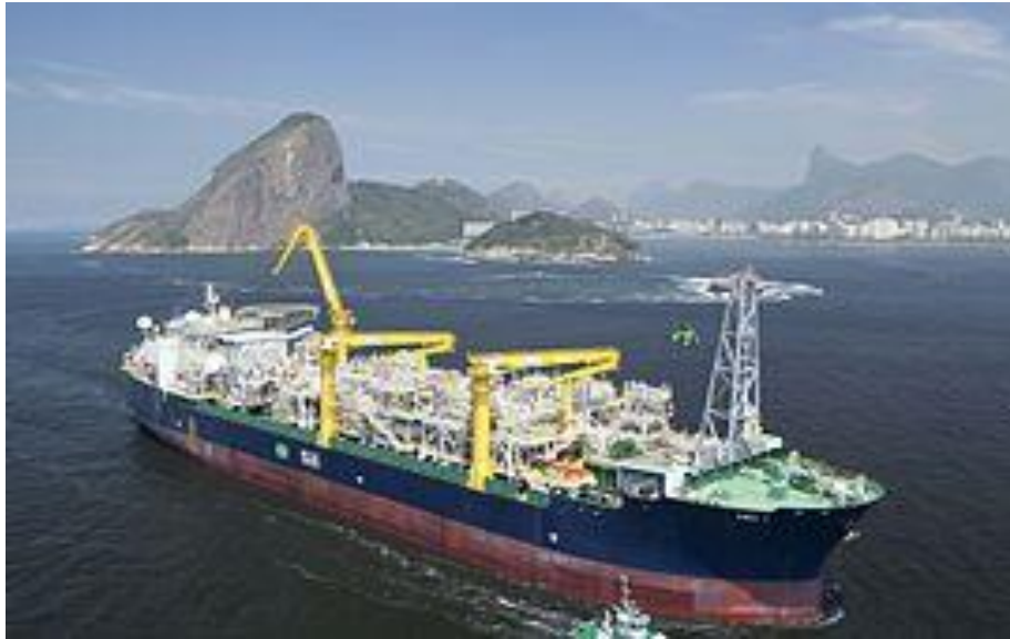
Figure 8: A tanker converted to an FPSO ship. An FPSO ship is similar to a tanker but it has additional piping and equipment on deck.
