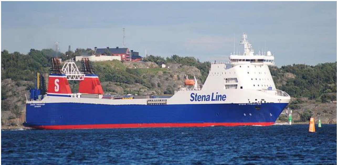
Figure 19: A Roll-On-Roll-Off Truck Carrier. These ships have a large ramp at the stern that closes watertight, and it may also have a bow door that hinges up so the trucks can drive out without turning around at the other end of the trip.
