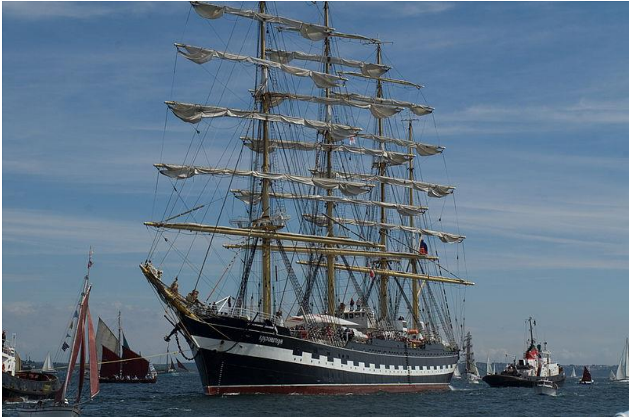
Figure 33: Russian Sail Training Ship Kruzenstern, one of the few operating 4-masted barques in the world. The painted gunports are for decoration
