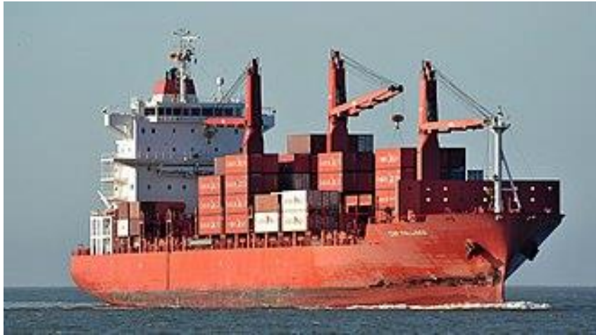
Figure 11: A fully loaded, self-loading/unloading containership. These ships operate between ports that do not have the large cranes shown in Figure 4.
