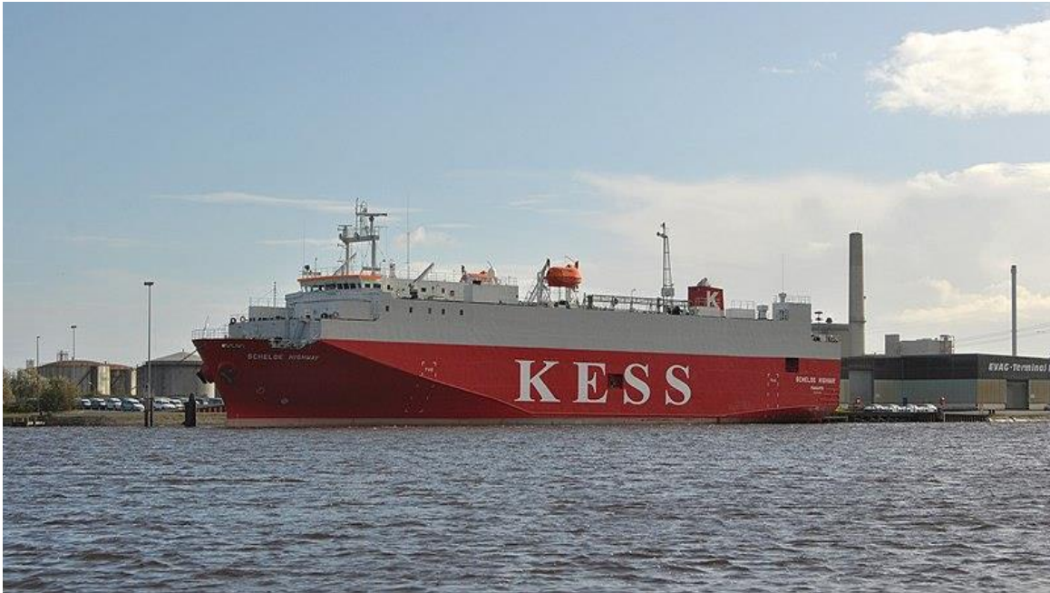
Figure 4: This is a Roll On-Roll Off car or truck carrier, which carries freight containers on trailers and/or cars that are driven onto and off the ship.
