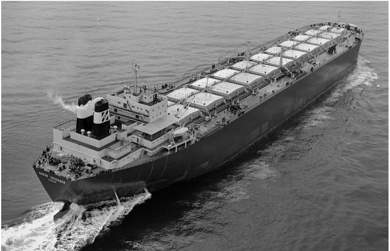
Figure 1: Bulk Carriers are distinguished by their multiple matches. This one is not capable of self-unloading and must tie up to a dock with loading/unloading cranes and conveyor belts
