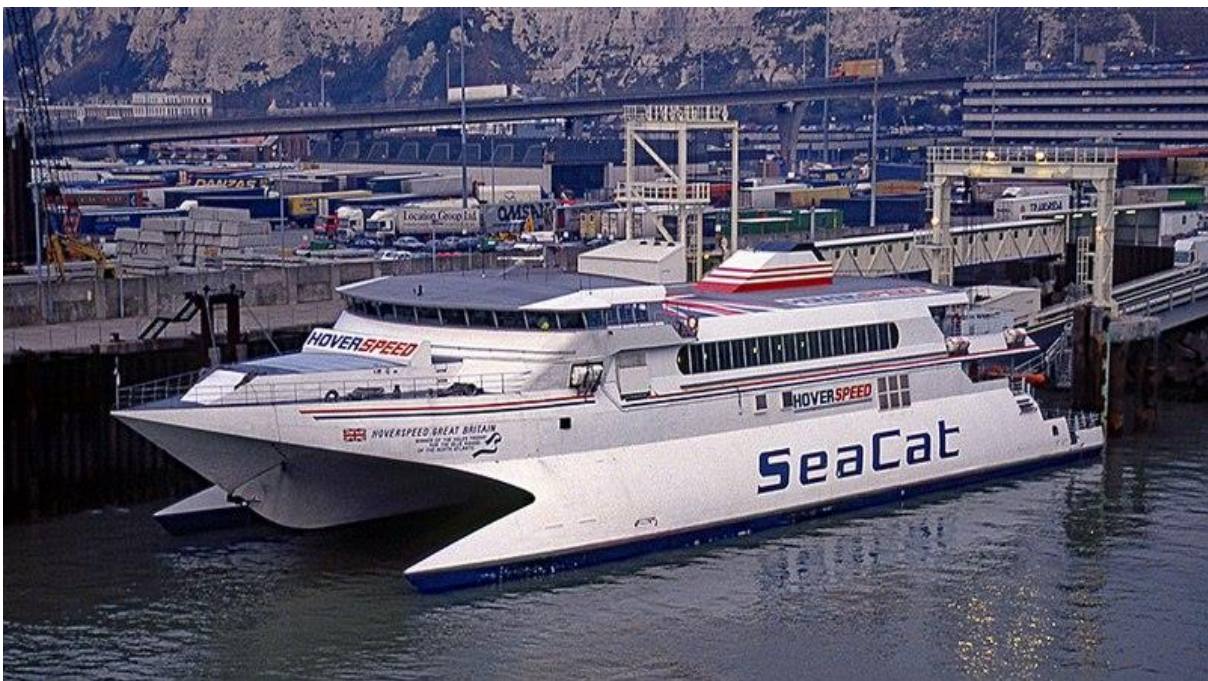
Figure 25: A Wave-Piercing Catamaran Ferry. The center hull breaks the bow wave, and the sidehulls pierce the wave like torpedoes while providing the buoyancy.
