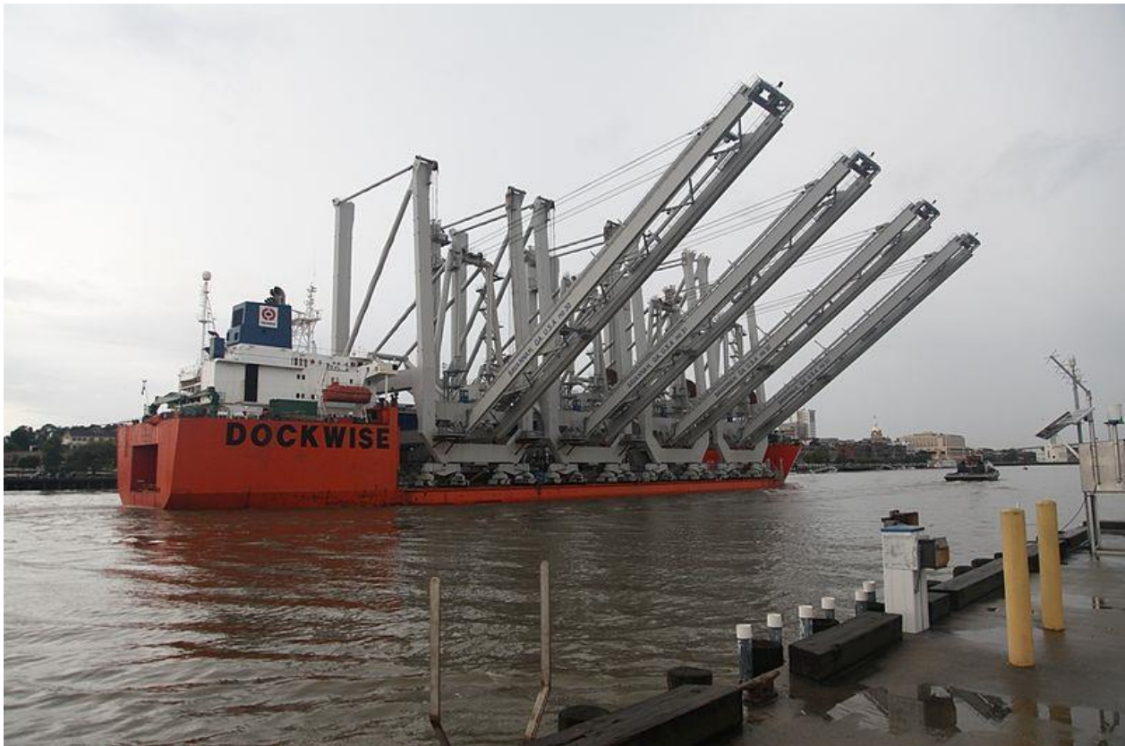
Figure 15: Another semi-submersible type carrying large container cranes to a port as cargo. This is a cargo that would make me nervous!
