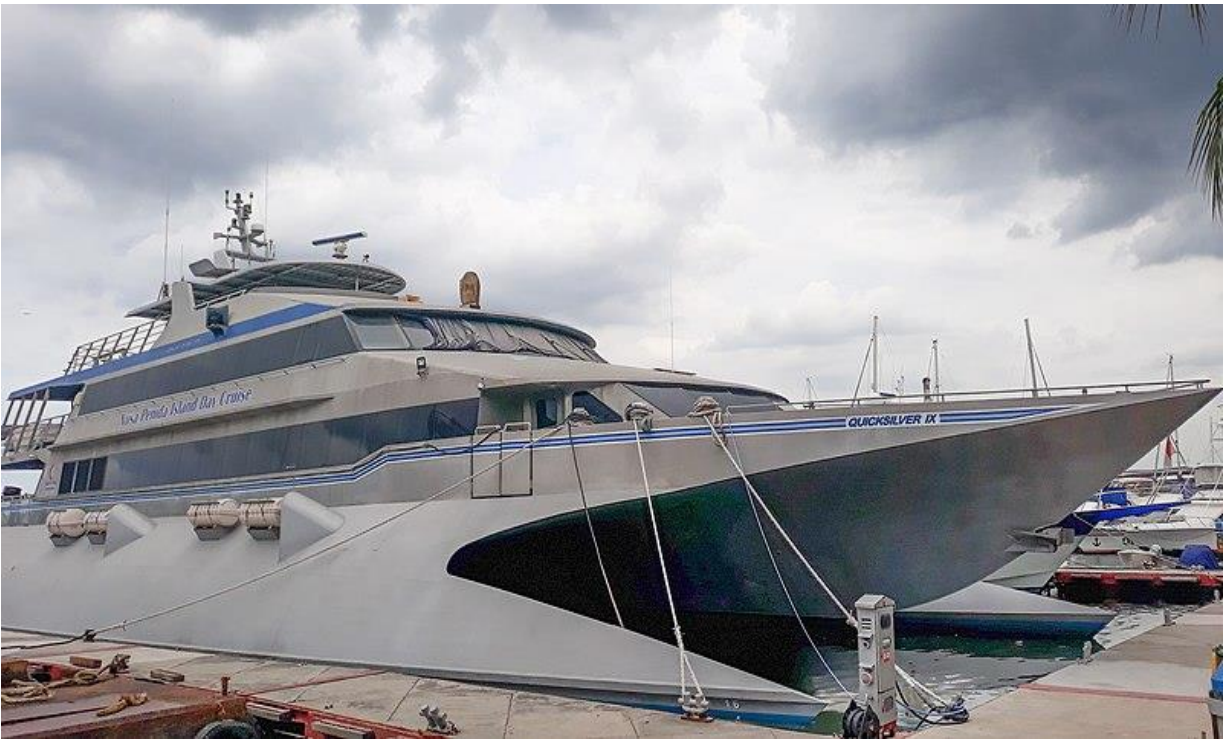
Figure 25: A Wave-Piercing Catamaran Ferry. The center hull breaks the bow wave, and the sidehulls pierce the wave like torpedoes while providing the buoyancy.
