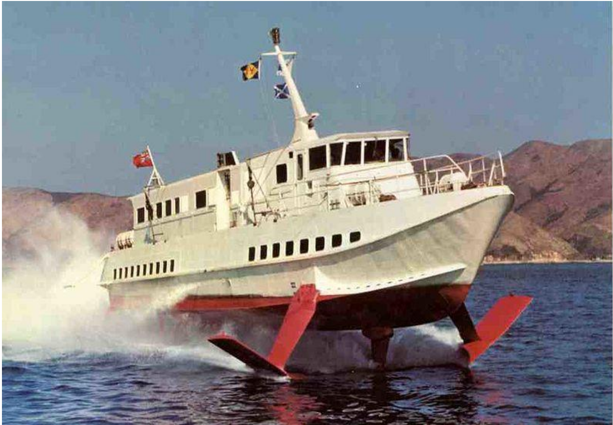
Figure 29: An old hydrofoil. These were popular in the 1960-1980's, but they have been mostly replaced by catamarans and wave-piercers.
