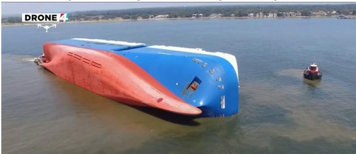
Figure 6: Car carrier Golden Ray aground and capsized. Note the high-speed hull lines and how they transition to a nearly cubical shape above the waterline.(courtesy News4 Jacksonville)
