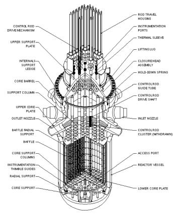
A Pressurized Water Reactor cut-away view. Loose part was in the bottom below the fuel and core support..
