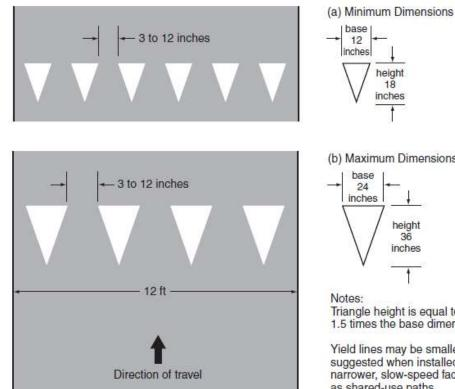
Figure 14. Recommended yield line layouts (MUTCD Figure 3B-16)
