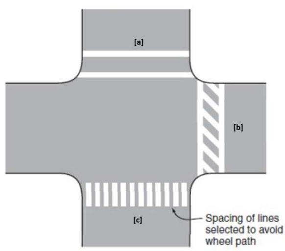
Figure 17. Examples of crosswalk markings (MUTCD Figure 3B-19)
