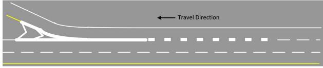
Figure 7. Wide dotted line exit lane drop marking
