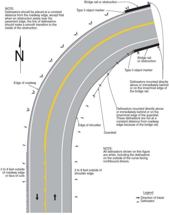
Figure 28. Examples of delineator placement (MUTCD Figure 3F-1)
