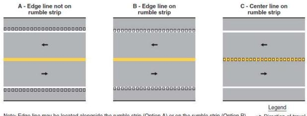
Note: Edge line may be located alongside the rumble strip (Option A) or on the rumble strip (Option B). → Direction of travel Center line markings may also be located on a center line rumble strip (Option C).
