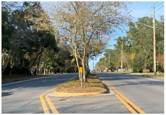
Figure 29. Yellow pavement color on raised median island separating traffic
