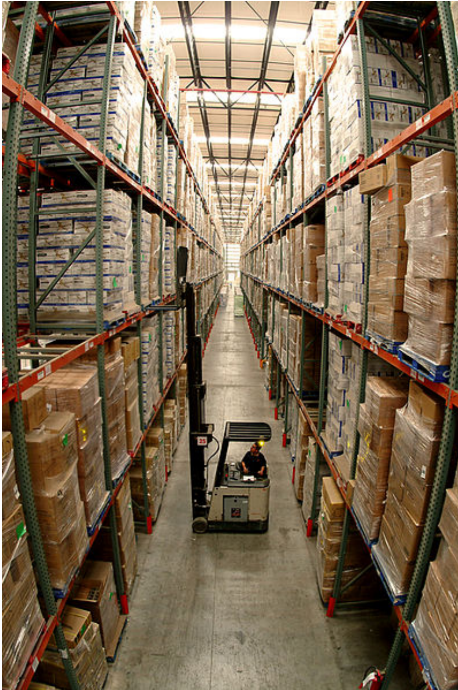
Fig. 25 - Stacker lift making a placement/retrieval of a pallet
