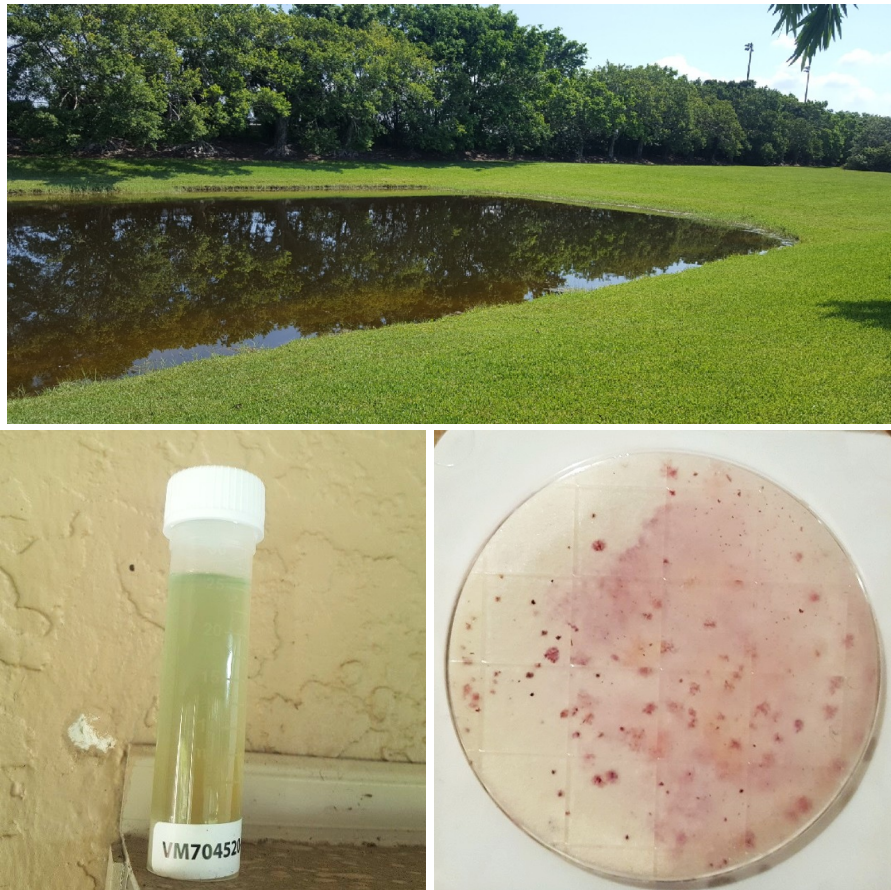
Figure 11: Pond in the author's backyard (top), Fecal Coliform Test with a positive result, and HPC Test with a count of approximately 100 CMU/ml.
