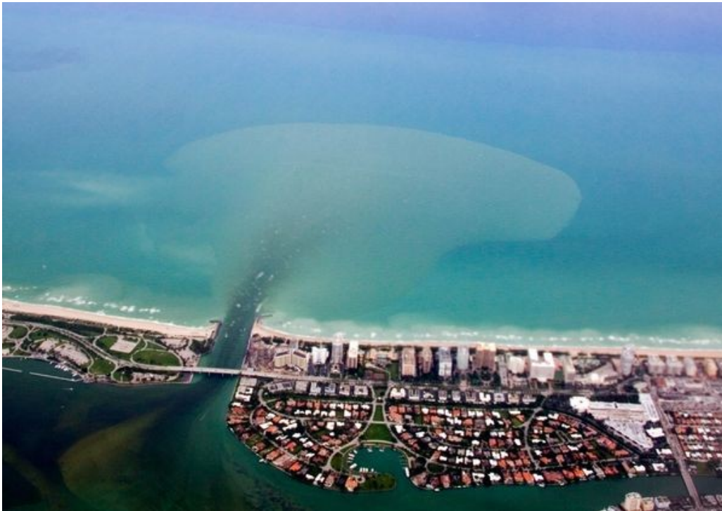
Figure 13: An example of an intercoastal port releasing brackish water into the ocean during low tide. The brackish water contains surface water from urban runoff, canals, rivers, and other sources that contain biological contaminants.
