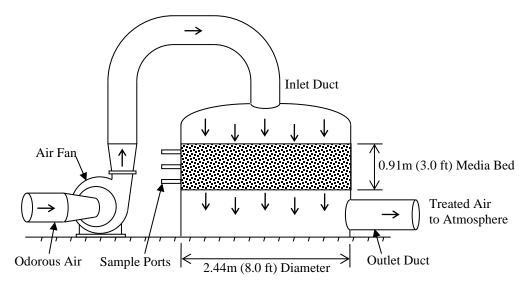
Figure 8: Schematic diagram of the activated carbon system.
