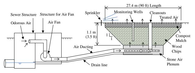
Figure 9: Schematic diagram of the biofilter bed system.
