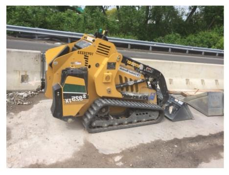
Walk Behind Rubber Tracked Loaders: With even lower profiles provide even more clearance than the skid steers and gain more access under existing bridges for reconstruction projects. Rubber Tracks allow for load distribution on and movement on loose graded No. 8 & 67 aggregate.
