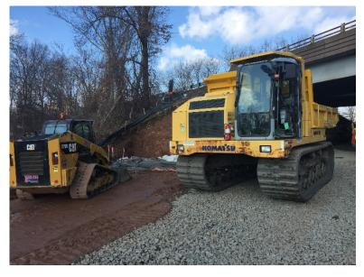
Tracked 360-degree Rotating Dumps: For restricted access bridge reconstruction projects, the 360-degree operation eliminates backing on long distances. Faster hauling and disposing of excavated material and delivery of backfill material. Tracks allow better load distribution and maneuverability in tight quarters.
