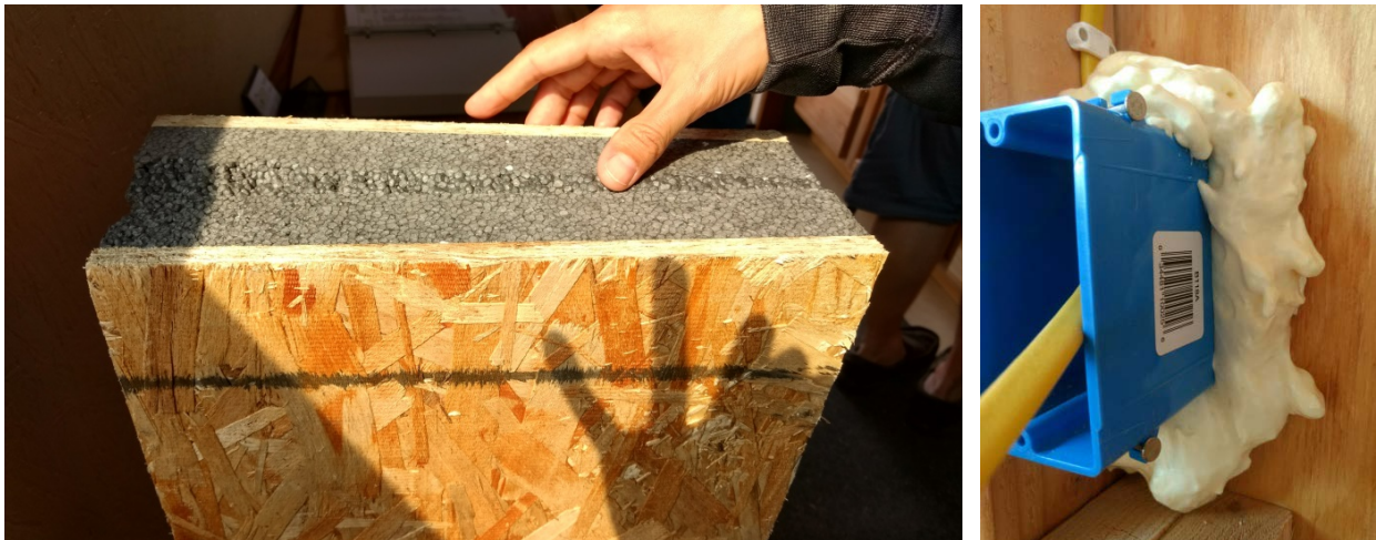
Left: A structural insulated panel (SIP), which sandwiches rigid foam insulation between structural sheathing. No studs or joists are needed between the structural sheathing so thermal bridging is avoided. SIPs can be used as wall or roof assemblies. After installation proper air sealing between each SIP piece is critical. Some companies are now making THOW with SIPs.
