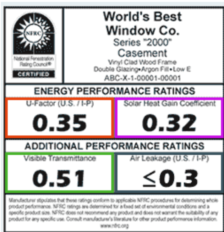
Figure 3: A National Fenestration Rating Council (NFRCC) energy performance label showing the U-factor, SHGC, visible transmittance, and air leakage testing results for a fictitious window (from NFRCC fact sheet). Energy performance label stickers should be on all new windows made in the United States.
