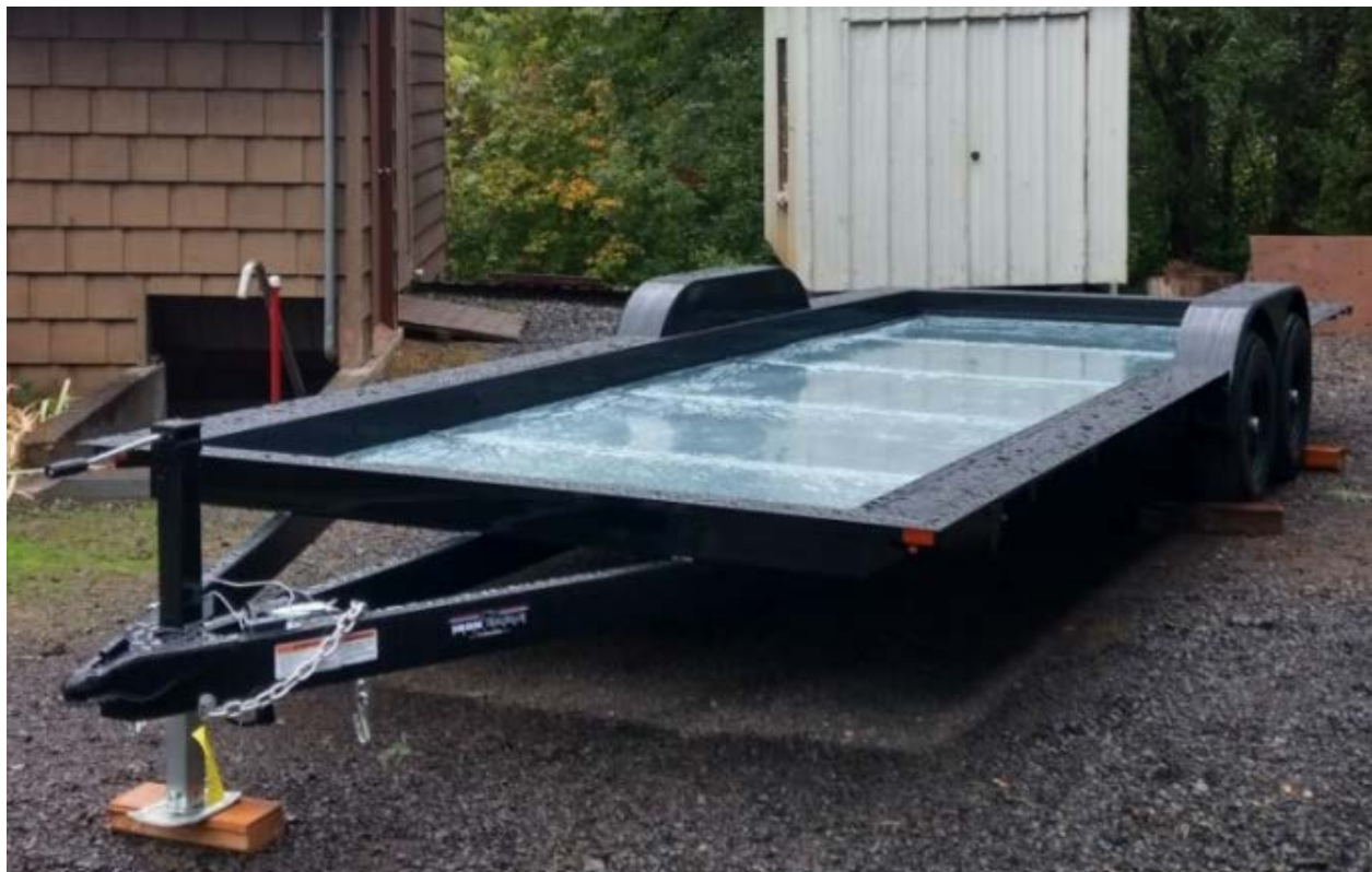
Tiny house specific trailer with galvanized sheet metal bottom pan
