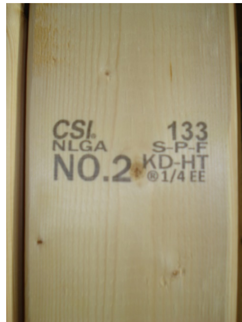
Right: 2x4 graded using the Canadian Softwood Inspection (CSI) standards, not the WWPA Standards. Regardless, the format is similar enough to tell it is No. 2 Spruce-Pine-Fir (SPF) that was kiln-dried (KD) and heat treated (HT) for export purposes. The 1/4 EE means the 2x4 has a 1/4 inch eased edge (round edge).
