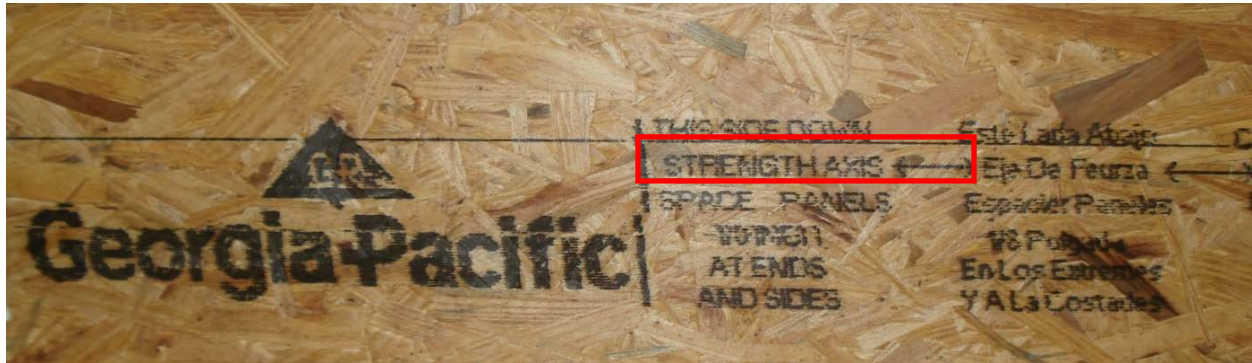
OSB with a stamp showing the strength axis direction
