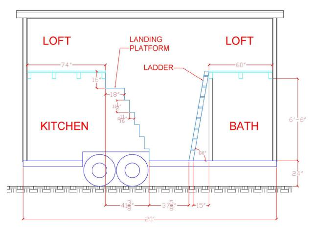
Figure 3: Example Stair and Ladder Access to Lofts
