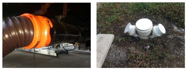
Left: A typical 3" diameter sewer connection on an RV. This hose has a "bayonet" style connection.
