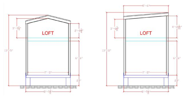
Figure 2: Two Common Sections for THOW
