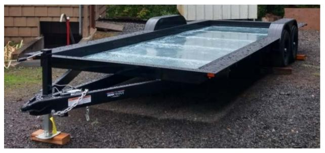
Tiny house specific trailer with galvanized sheet metal bottom pan to protect the floor assembly from water and insects
