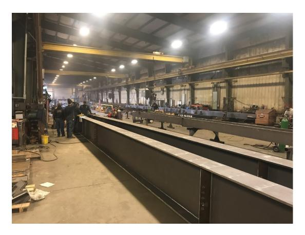
The raw steel will be delivered to the fabrication yard. The pieces will be brought into the shop for cutting, welding, and cleanup. Each piece will be given a distinct piece mark and erection/bolt up drawings will be provided to detail the sequence and layout each piece must be placed in the structure to ensure proper fit. Protective and architectural coatings will be shop applied as a last step in the fabrication process.
