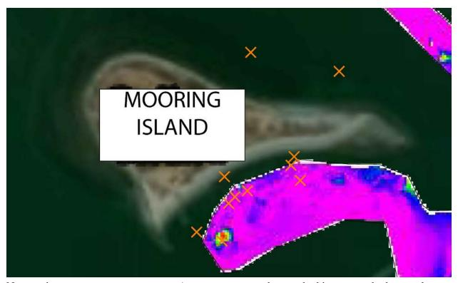
Next up is our magnetometer survey. As you can see on the attached image, we had a couple more targets come up (signified by the x). As with the side-scan survey, these targets represent areas that require further investigation.
