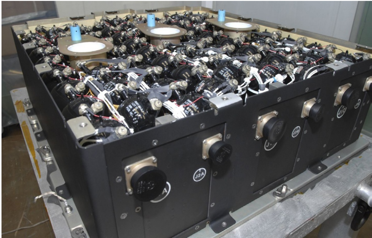
Figure 2.4: Hubble Space Telescope New Battery Module Assembly [Reprint from source: NASA @ nasa.gov]
