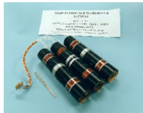
Rover Primary Batteries
