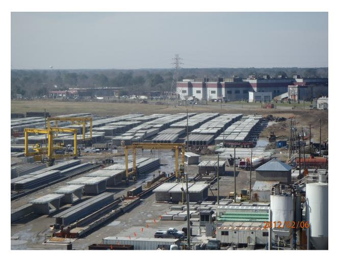
After a day's production, the previous day's match cast segment is ready to be finished and set for storage. Depending on the design, some segments can be lifted and placed in storage prior to any post-tensioning. This will be a factor of strength gained during
