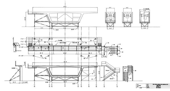
Example of Pier or Expansion Segment Formwork Drawings
