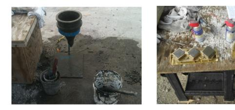
Grout cubes and flow tests are performed by the QC department to ensure the grout meets the specifications and the operations are acceptable.
