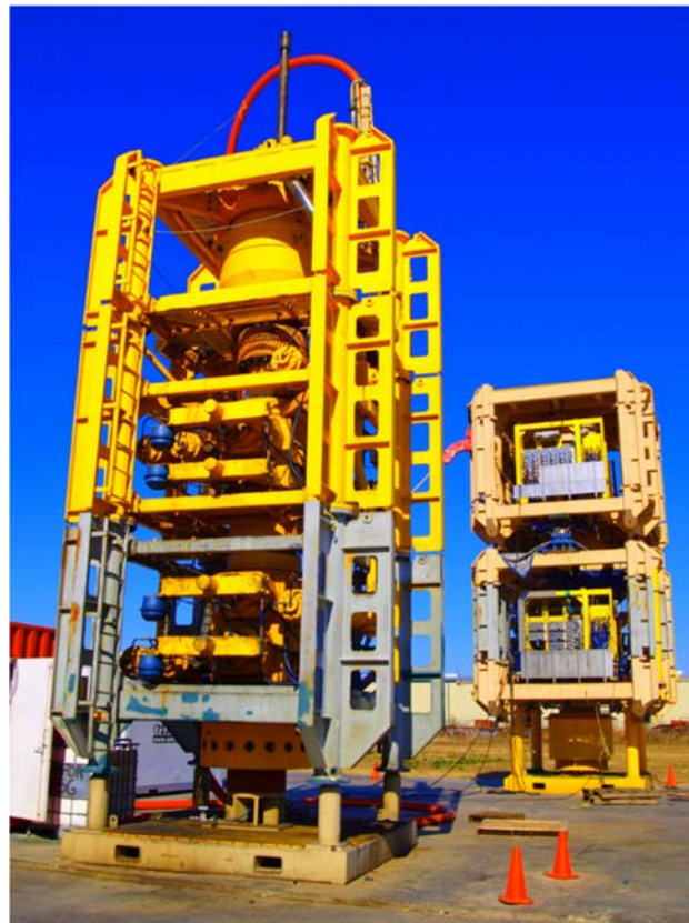
Blowout preventer stack
