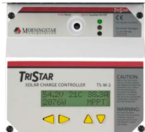
TS-M-2 Monitor Meter on Morningstar TriStar MPPT-60 charge controller
