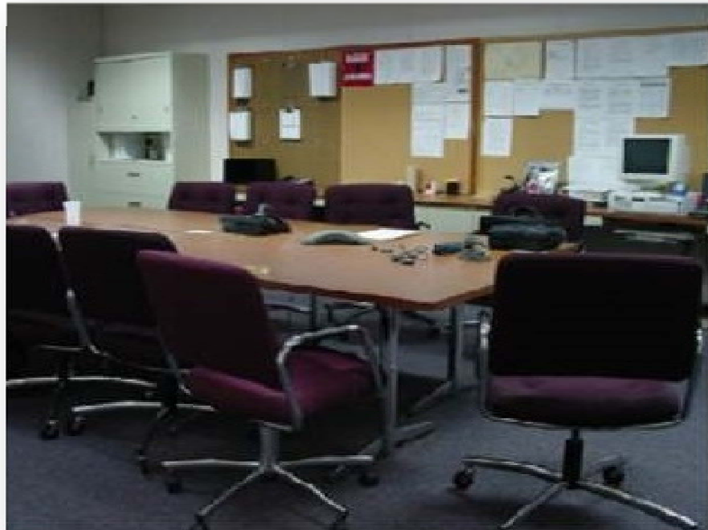
Figure 9a – Space lit with two (2) 4100°K fluorescent lamps per fixture
