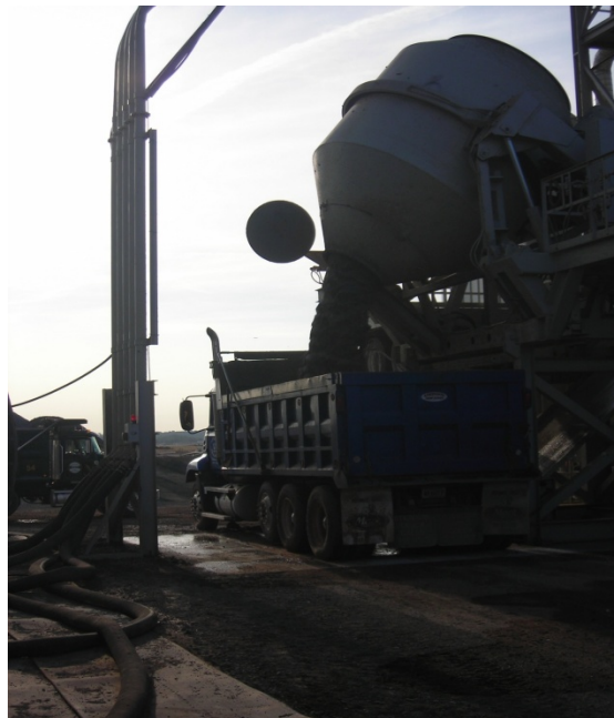
Central Drum Concrete Plant with extra cement storage next to a cement treated aggregate Pugmill Plant at an airport apron concrete paving site. Cement treated aggregate was used for base course material under 16" of concrete pavement.
