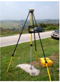
Traditional mapping grade receiver Survey grade GPS antenna mounted on tripod over a geodetic survey mark Source: NOAA
