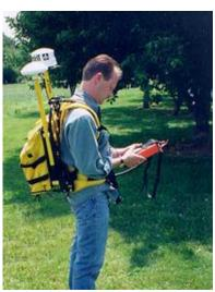
Backpack mounted GPS roving antenna and receiver unit Source: NOAA
