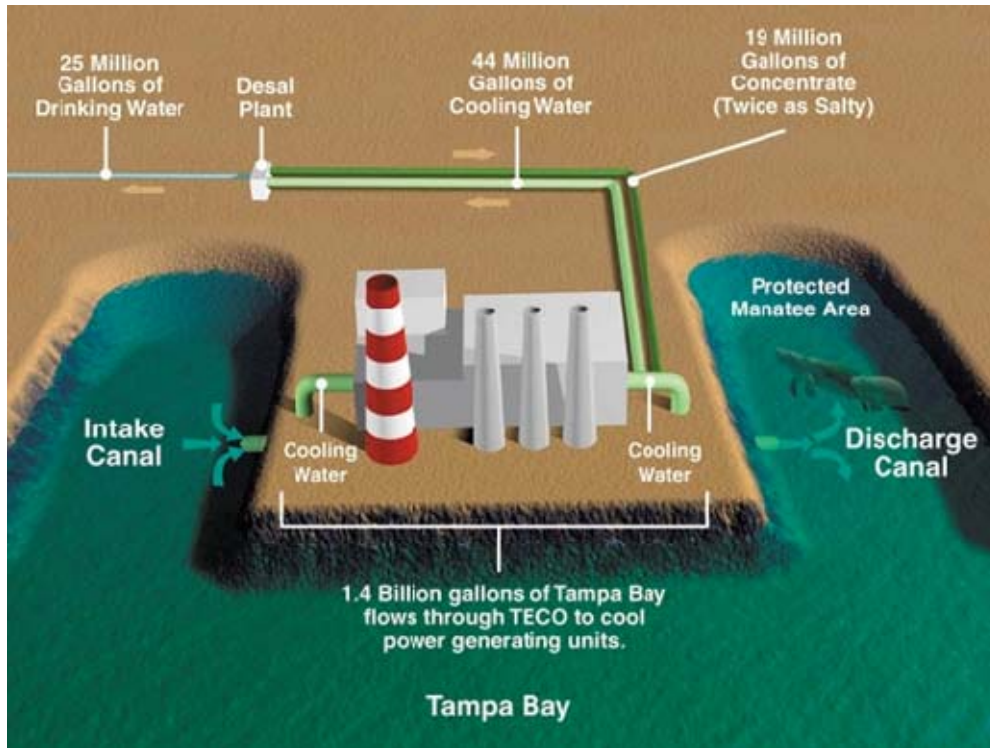
Figure 7 – Tampa Bay SWRO Plant Collocation Schematic
