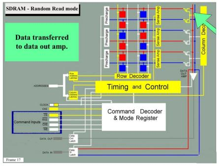
The differential signal from the selected bit line pair is coupled to the internal data lines and sent to the DATA OUT AMP.
