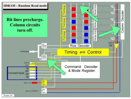
The bit lines precharge and the column-related circuits turn off.
