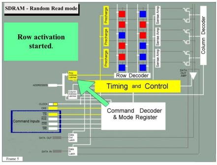
The Row Address Latches sense the address input voltage levels and generate and store internal addresses that are sent on internal address lines to the Row Decoder.
