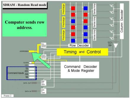
As the first step in starting an ACTIVE operation, the computer sends row addresses to the Address pins of the SDRAM.
