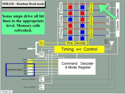
and rewrite the information into the memory cells that initially provided it, thus refreshing the memory cells on the selected word line.
