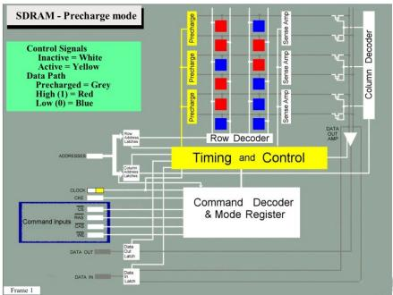
In the Precharge mode, the SDRAM is idle and awaiting inputs and a command to start an operation.
