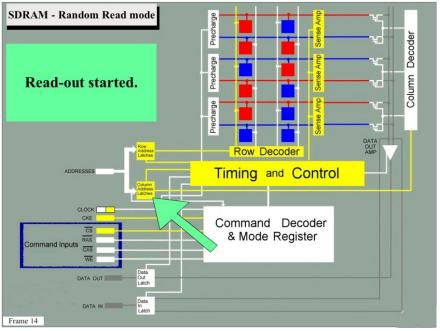
The Column Address Latches sense the address input voltage levels and generate and store internal addresses that are sent on internal address lines to the Column Decoder.
