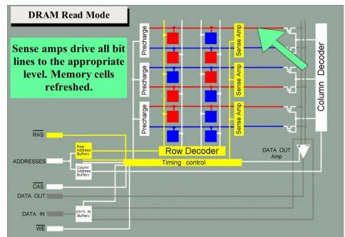
and rewrite the information into the memory cells that initially provided it. As mentioned above, this rewriting is called "refreshing", and must be done periodically to every memory cell on the chip.
