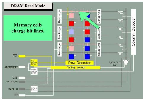
The information stored in those memory cells, represented as electrical charge or lack of charge, slightly changes the voltage on those bit lines. Therefore, there will be a voltage difference between each bit line and its corresponding complement bit line (the bit line pair), caused by the information in the memory cell now attached to that bit line.
