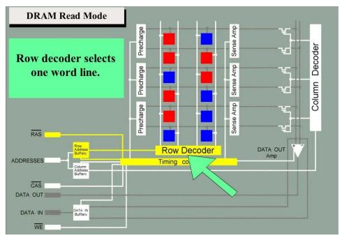
Based on the internal addresses applied to it, the Row Decoder identifies and activates the appropriate word line.
