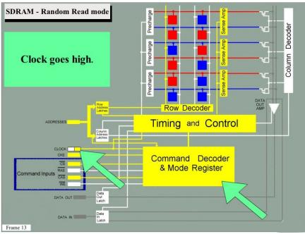
The logic states of the 4 command inputs, as well as the address inputs, are sampled and sent to the Command Decoder and Column Address Latches respectively when the Clock goes high.
