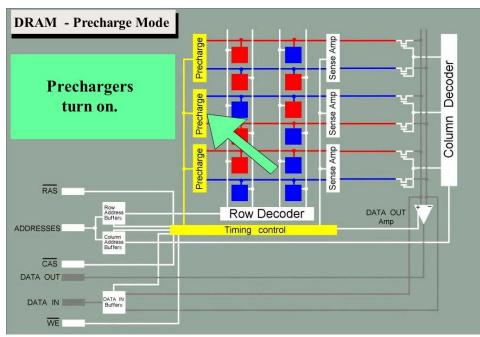
The bit line Precharge circuits are turned on.
