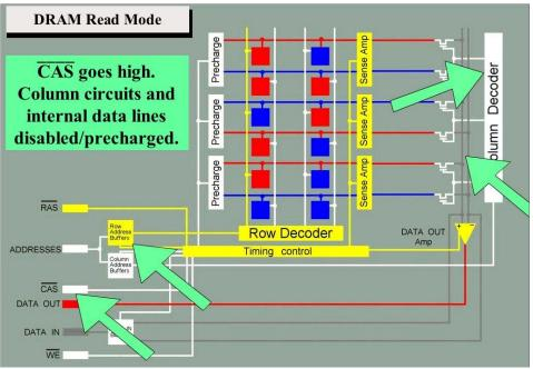
To start the recovery, CAS/ goes high, thus allowing column circuits and internal data lines to be recovered to their precharged levels.
