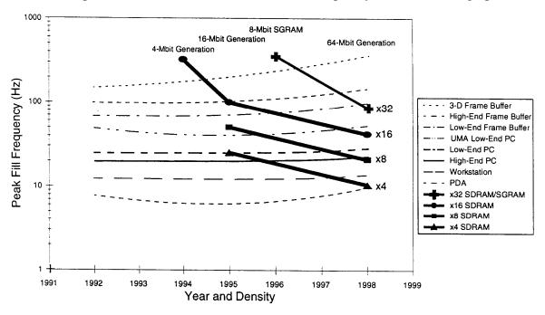
The impact of the SDRAM architecture on fill frequency is shown in the graph below.
