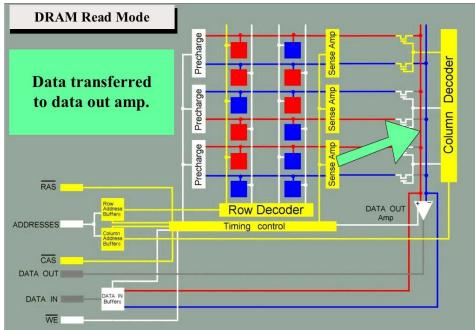
The differential signal from the selected bit line pair is coupled to the internal data lines.
