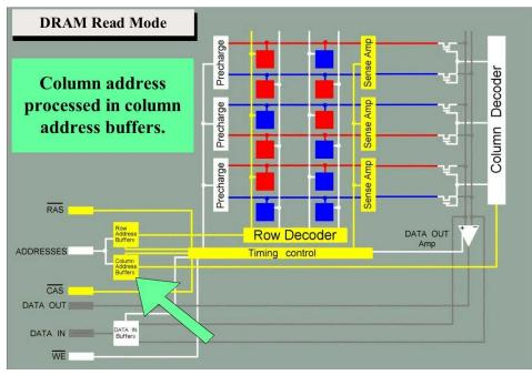
The Column Address Buffers sense the address input voltage levels and generate internal addresses that are sent on internal address lines to the Column Decoder.
