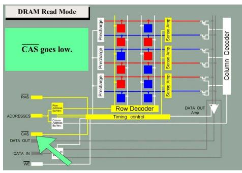
Then a signal called CAS/ (pronounced CAS-Bar) is applied to the memory<sup>11</sup>, thus gating the voltages on the Address Pins into the Column Address Buffers.
