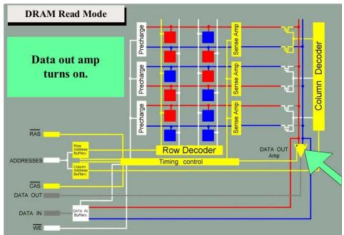
The signal on the internal data lines is amplified by the DATA OUT Amp.
