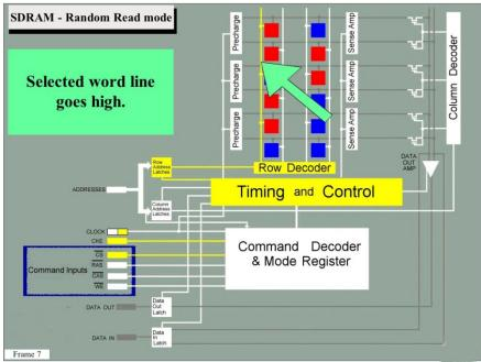
When the word line is activated, all of the memory cells attached to that word line are connected to their respective bit lines.
