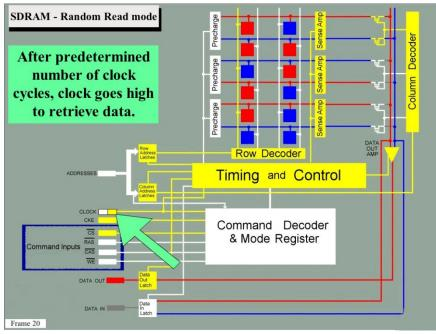
One cycle before the CAS Latency expires, the rising clock edge starts the read-out process from the Data Out Latch. Before the next rising clock edge (marking the end of the CAS Latency time), valid data appears at the DATA OUT pin.
