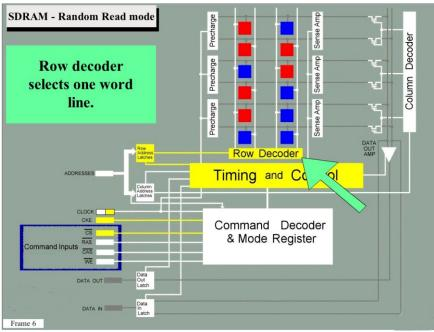
Based on the internal addresses applied to it, the Row Decoder identifies and activates the appropriate word line.
