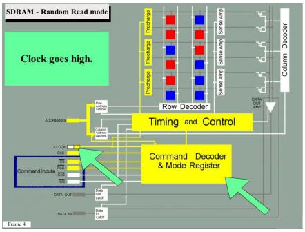
The logic states of the 4 command inputs, as well as the address inputs, are sampled and sent to the Command Decoder and Row Address Latches respectively when the Clock goes high.
