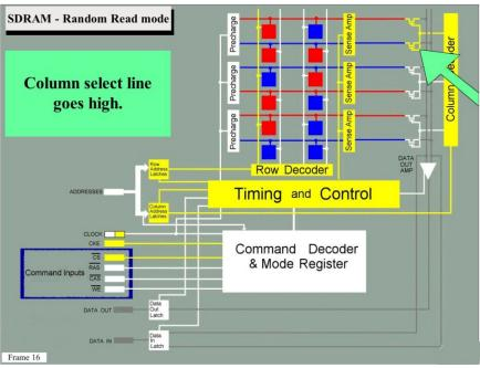
The Column Decoder selects and drives the Column Select line high.
