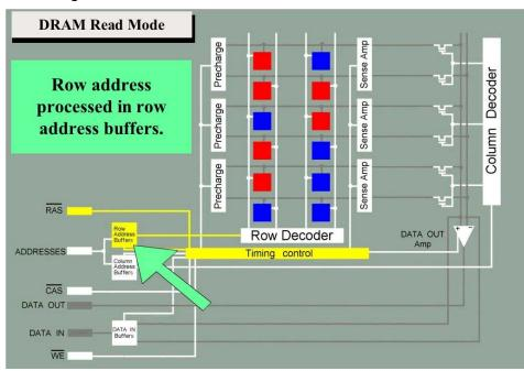
The Row Address Buffers sense the address input voltage levels and generate internal addresses that are sent on internal address lines to the Row Decoder.
