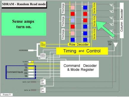
The bit line Sense Amplifiers amplify the voltage difference on each bit line pair,
