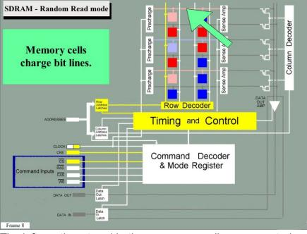
The information stored in those memory cells, represented as electrical charge or lack of charge, slightly changes the voltage on those bit lines. Therefore, there will be a voltage difference between each bit line and its corresponding complement bit line (the bit line pair), caused by the information in the memory cell now attached to that bit line.
