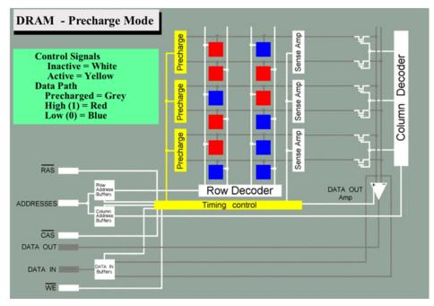
To illustrate memory operation, suppose that the memory is to be instructed to read the data in the top left cell and convey it to the output.
