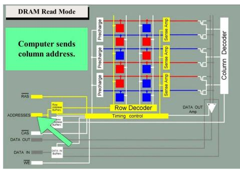
While the sense amplifier is operating, new voltages representing the address of the desired column are applied to the Address Pins.
