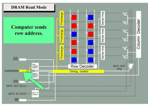
First, voltages representing the address of the row to be selected are applied to the Address Pins.
