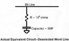
In the actual case, the Transistor remains very slightly on. Thus the charge on the Capacitor leaks off to the Bit Line.
