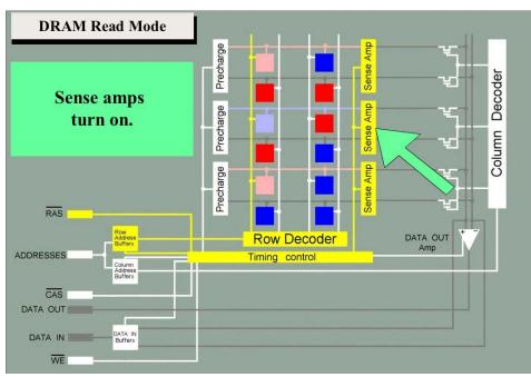
The bit line Sense Amplifiers amplify the voltage difference on each bit line pair,
