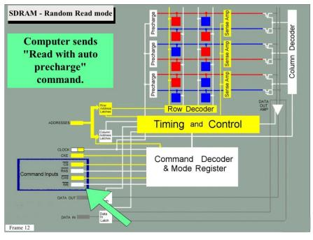
"Read with auto precharge" means that data will be read from the selected memory location, then the memory will be precharged so it is returned to the idle state.
