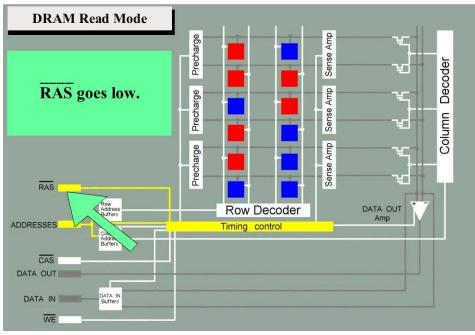
Then a signal called RAS/ (pronounced RAS-Bar) is applied to the memory, thus gating the voltages on the Address Pins into the Row Address Buffers.
