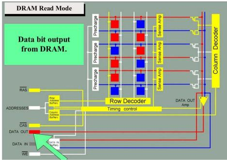
The output of the DATA Out Amp appears as valid data at the DATA OUT pin of the DRAM.
