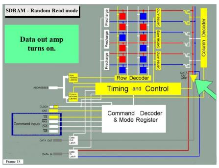
The signal on the internal data lines is amplified by the DATA OUT AMP.
