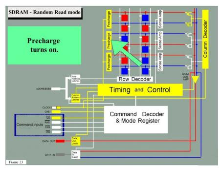
the bit line Precharge circuits are turned on.
