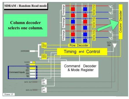
Based on the internal addresses applied to it, the Column Decoder is now activated and selects the desired column.
