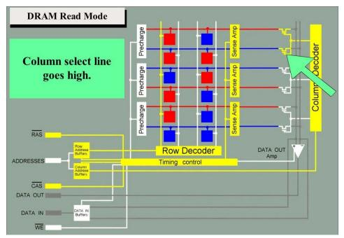
The Column Decoder selects and drives the Column Select line high.
