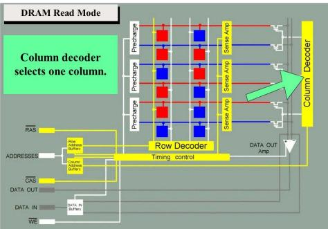
Based on the internal addresses applied to it, the Column Decoder is now activated and selects the desired column.
