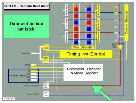
The output of the DATA OUT AMP is sent to the Data Out Latch. Note that, unlike in the DRAM, valid data does not appear immediately at the DATA OUT pin of the SDRAM.
