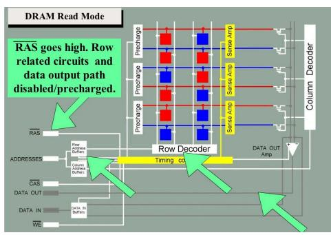
Then RAS/ goes high, first allowing the row circuits and data output path to be recovered to their precharged levels.
