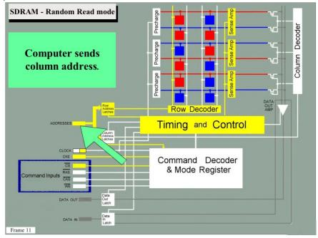
Another operation, as tabulated in the SDRAM COMMANDS table, can be initiated. Assuming we want to do a READ operation, the computer sends new voltages representing the address of the desired column to the Address Pins.
