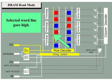
When the word line is activated, all of the memory cells attached to that word line are connected to their respective bit lines.
