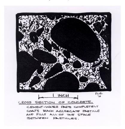
The aggregates used in making concrete are hard, inert materials. They have inert chemical properties. They just take up space. Aggregates compose about 75% of the
