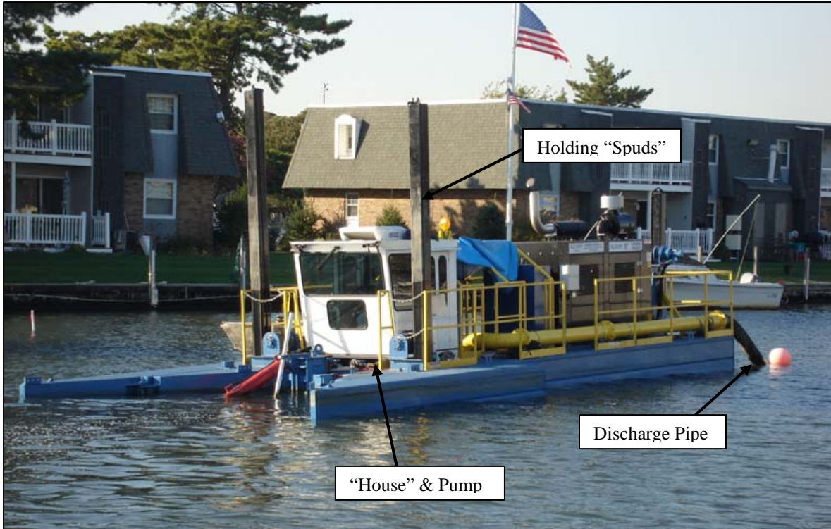
Figure 1: Small Hydraulic Dredge (Photo courtesy of Ellicott Dredges, LLC)
