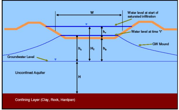
Figure 4: Saturated Infiltration & Groundwater Mounding
