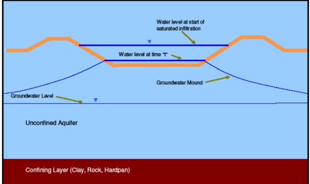
Figure 3: Saturated Infiltration & Groundwater Mounding
