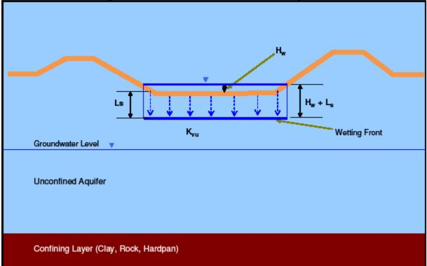
Figure 2: Unsaturated Infiltration & Wetting Front
